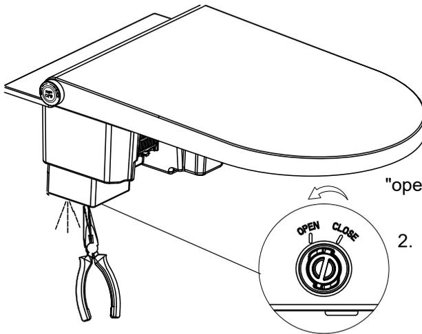
1. Hold the plug with the tipper , turn to "open" , and pull out . It will start to drain .
